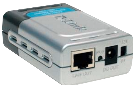
Splitters, such as this D-Link PWL-P50, allow conventional client devices to draw power from the network. The data and power on the PoE cable are separated and fed respectively to the unpowered network jack and DC power socket at the front of the device. This model allows you to choose between a 12v supply at a maximum 1amp or 5v at up to 2.5amp. The power lead needs to be wired for the correct polarity for the device you are using
